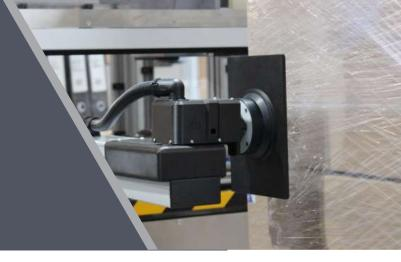
Introducing the Vector, a low maintenance high performance tertiary pallet labeller, capable of printing up to four labels on three sides with two pallet stop positions. The Vector pallet labeller completes Videojet's coding portfolio, enabling customers to benefit from joined-up coding solutions across primary, secondary and tertiary operations paving the way for the factory of the future.
