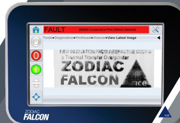
Checking system, iAssure™, detects bad prints
