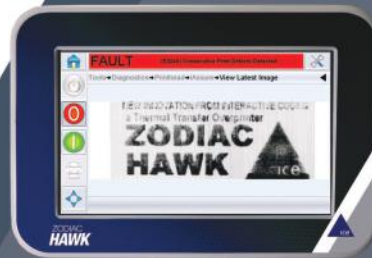
Checking system, iAssure™, detects bad print
