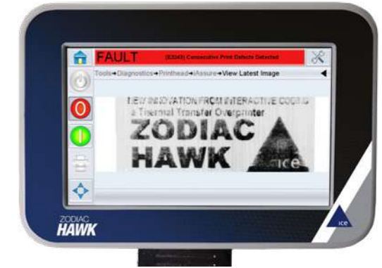
Checking system, iAssure™, detects bad prints
